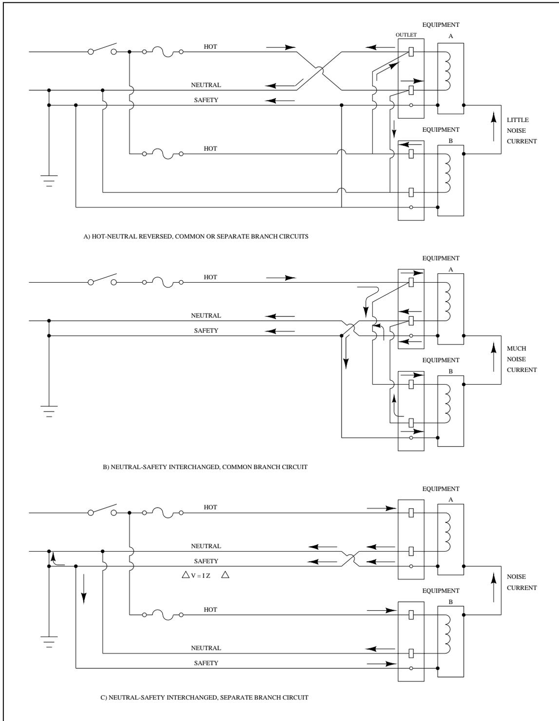
Figure 4-9. Noise problems resulting from improper wiring
