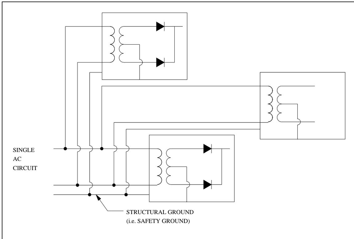
Figure 4-4. Basic grounding of a clustered system
