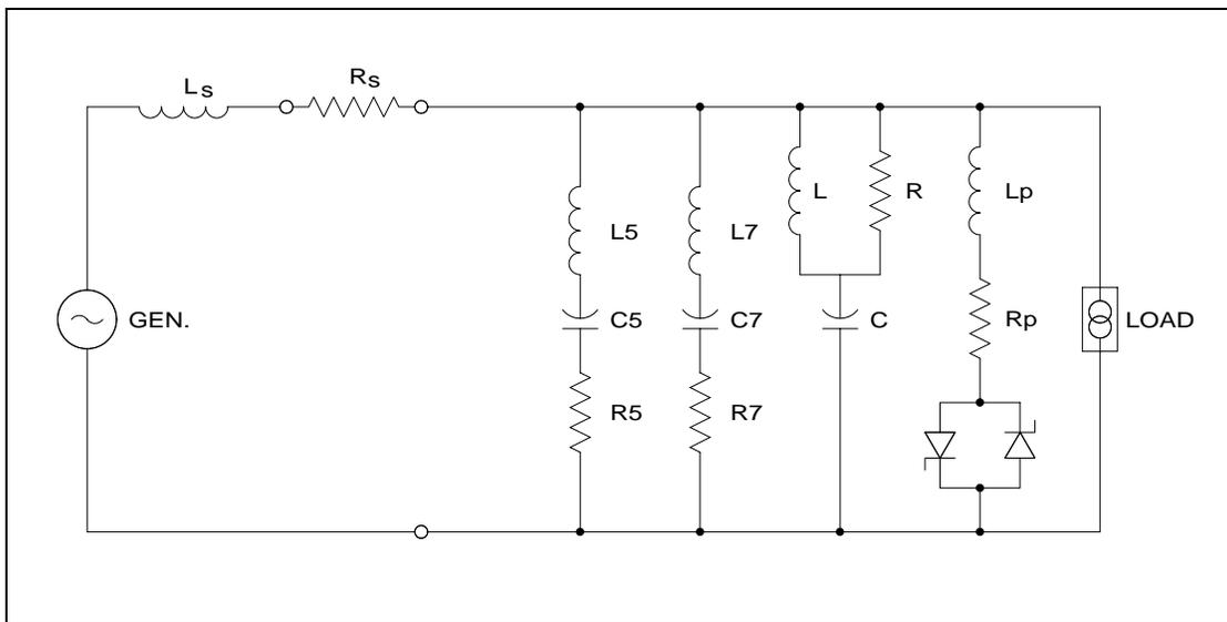
Figure 5-3. Tuned passive filter with static VAR control
