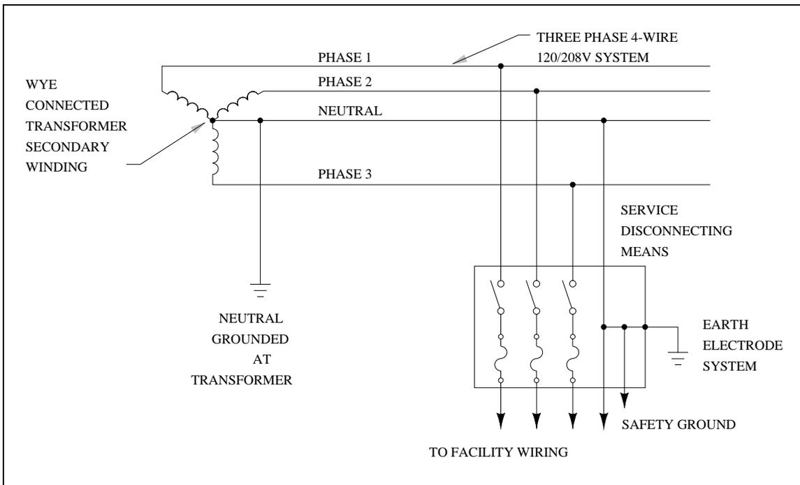
Figure 4-7. Three phase 120/208 Vac power system ground connections
