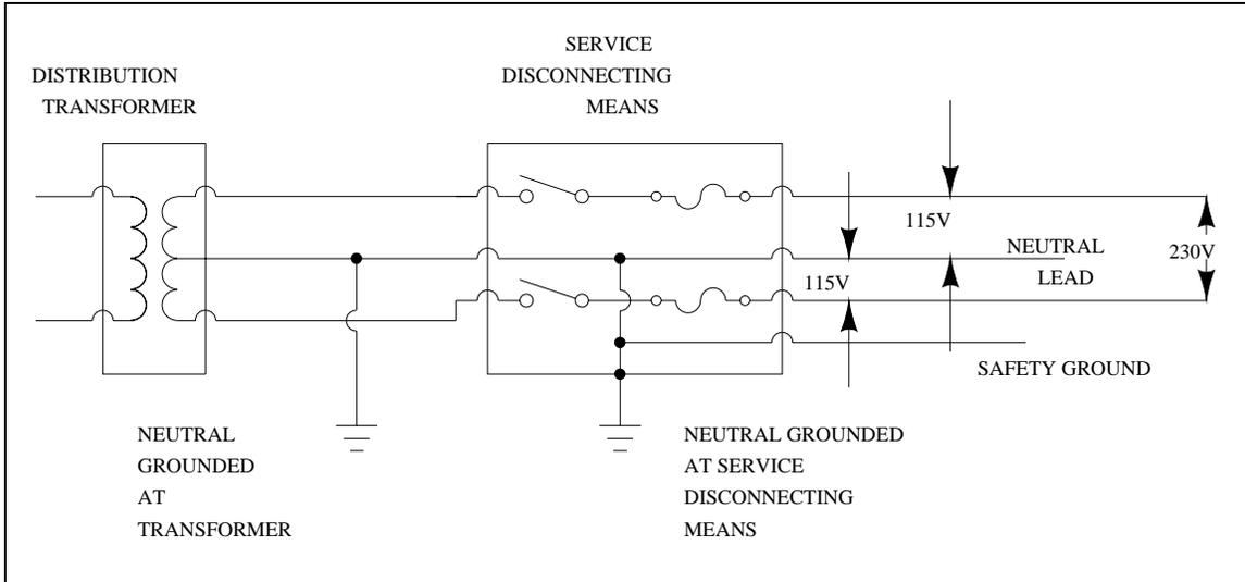
Figure 4-6. Single phase 115/230 Vac power ground connections
