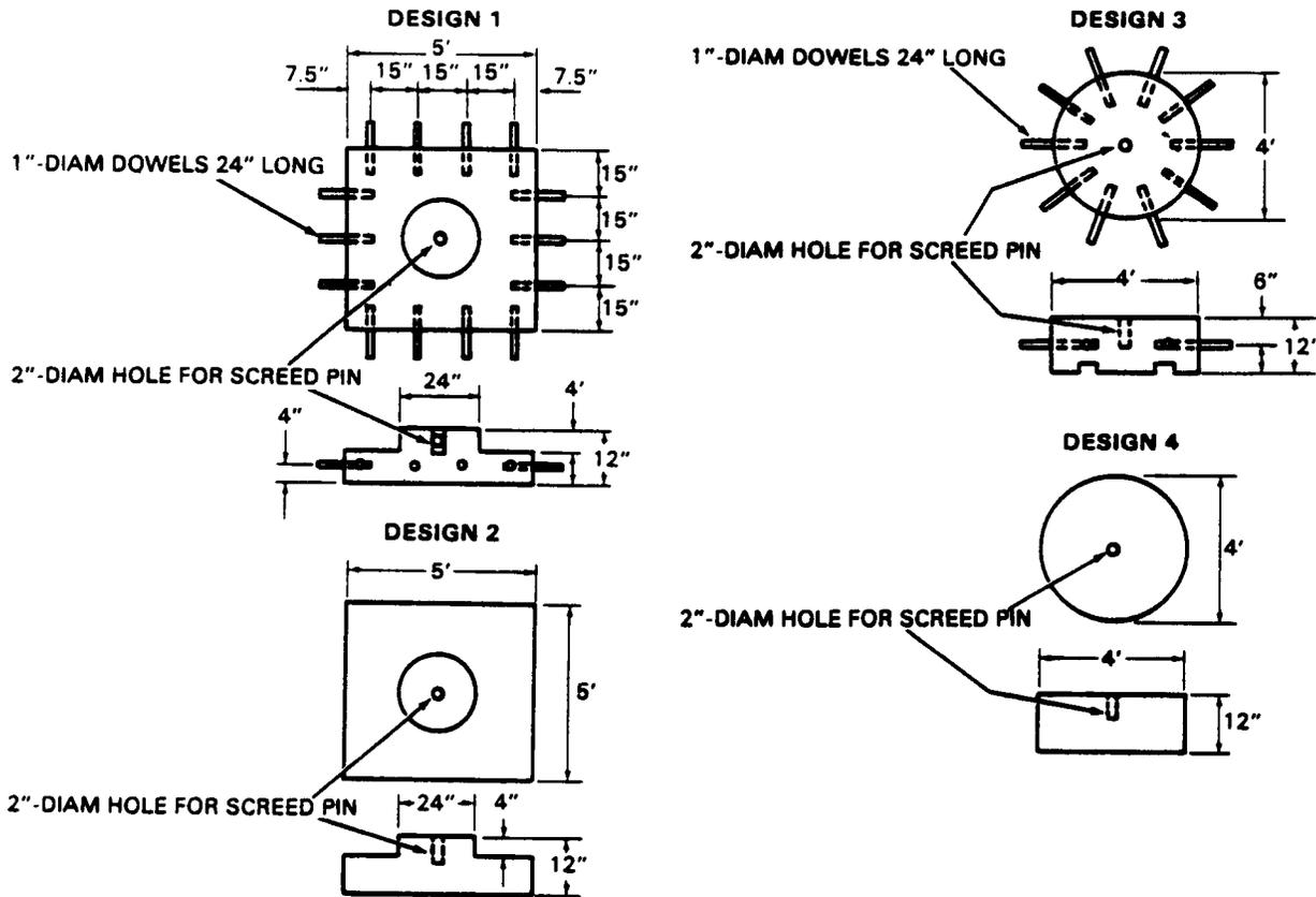
Prepare the center of the crater so that the surface of the prefabricated concrete pedestal is even with the surface of the runway pavement (see Figure B-4). This is best accomplished with a string line.
