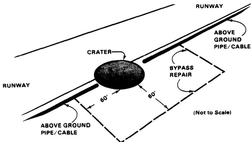
**FIGURE 7-2. BURIED CABLE BYPASS
