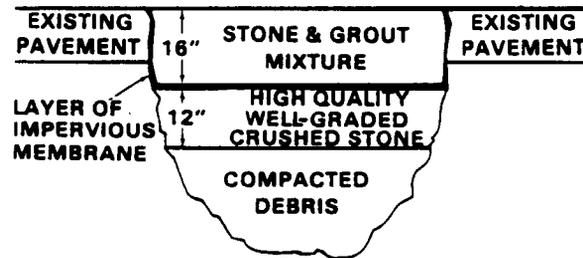
Clean the edges of the crater thoroughly and place a layer of sand approximately 1 foot wide by 1 to 2 inches deep around the entire inside of the crater. This is to prevent seepage of the grout around the edge of the crater.
