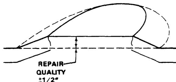
The instruments needed for surface roughness checks are two upheaval marker posts, a string line (see Figure A-2), and a change of slope straight edge (see Figure A-3). To determine the amount of upheaved pavement to break out--
