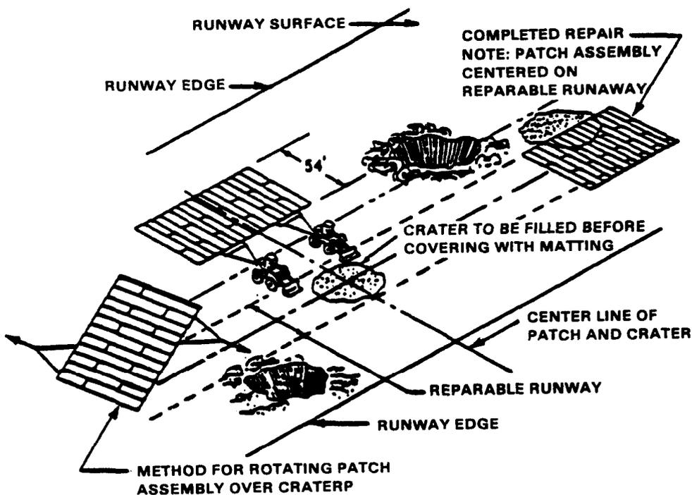
FIGURE D-4. PATCH ASSEMBLY - METHOD B
