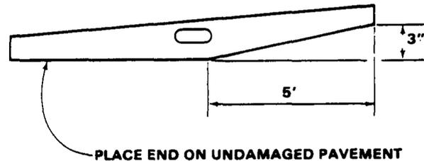
exceed 1 inch. These flatness checks should be made along three lines parallel to the MOS centerline. One line is along the MOS centerline (or along the centerline of the repair if the whole repair is on one side of the MOS), and the other two are halfway between this centerline and the edges of the crater.
