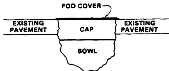
In preparing the bowl, all standing water must be removed from the crater bottom by the most efficient means available. This is necessary to allow for proper compaction of subsequent fill layers and to avoid an excessive settlement of the cap. Pneumatic pumps are ideally suited for water removal.
