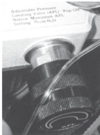
*Figure 2-1. Typical adjustable pressure-limiting valve.*
