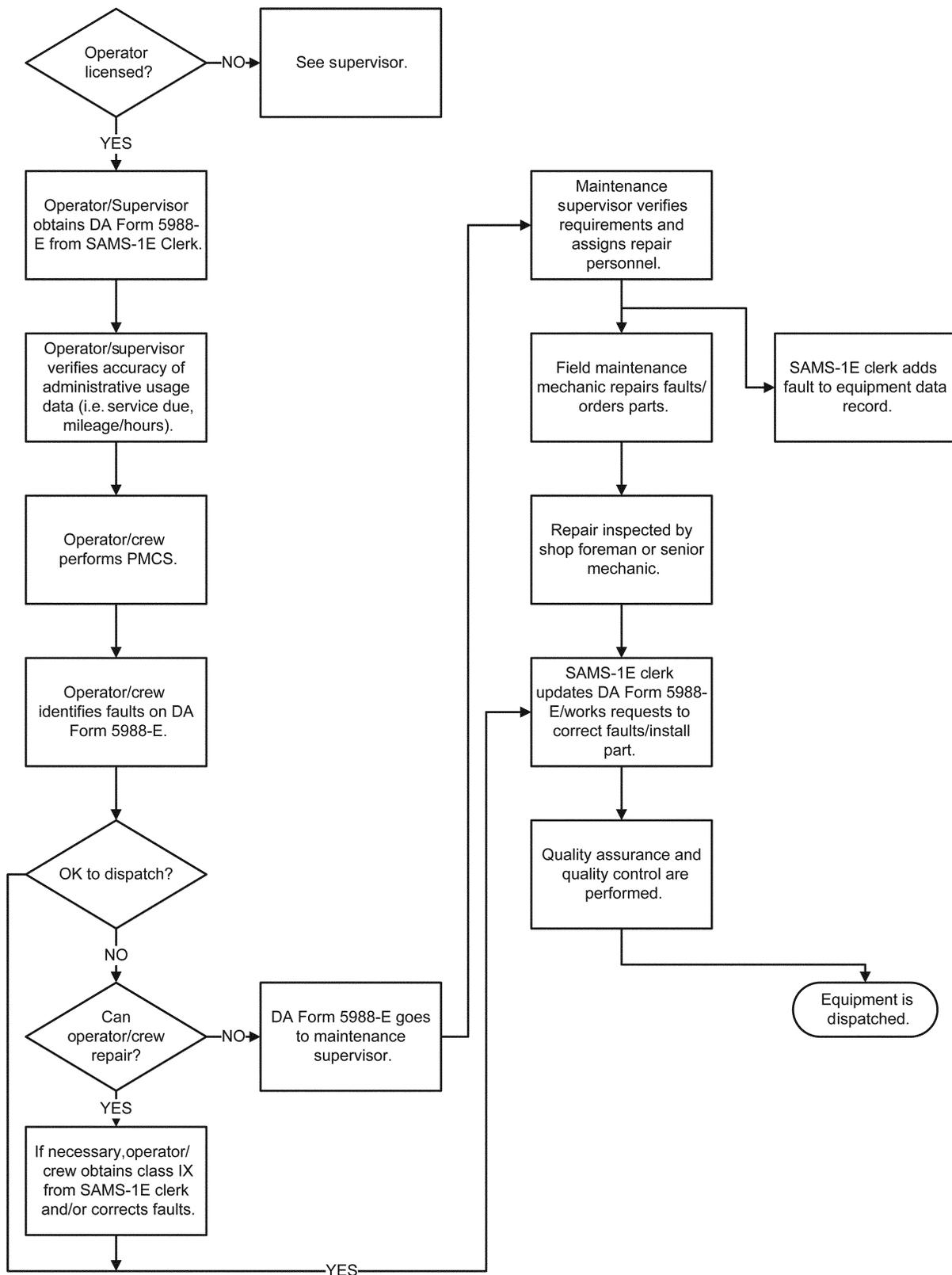
Figure 3-1. Equipment dispatch flowchart
