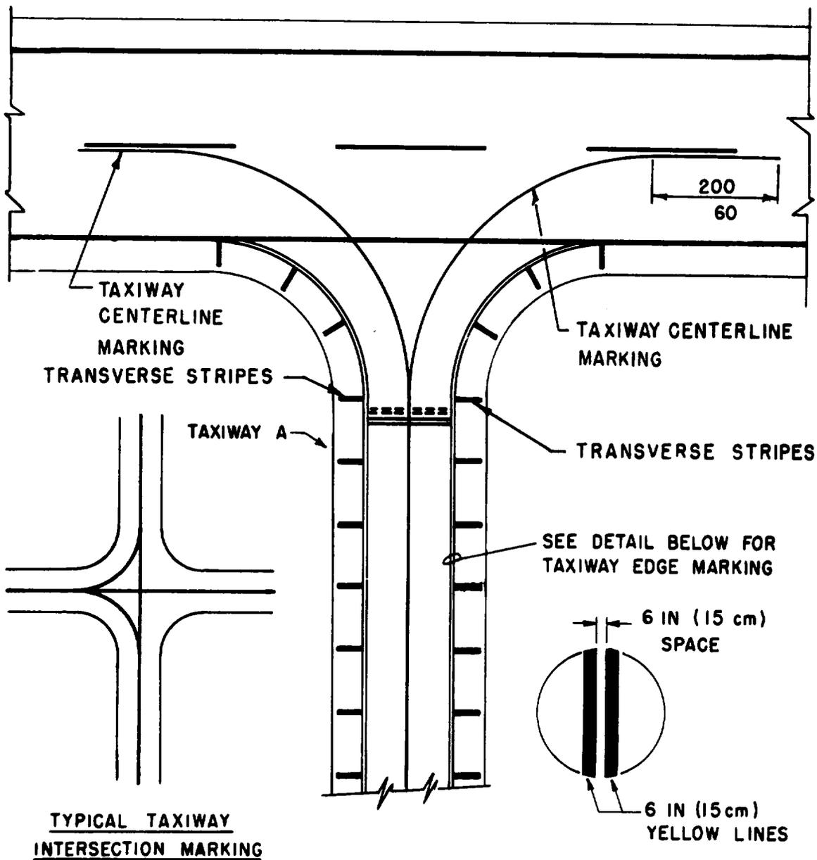
Figure 2-6. Taxiway/runway intersection marking. (Sheet 2 of 2).
