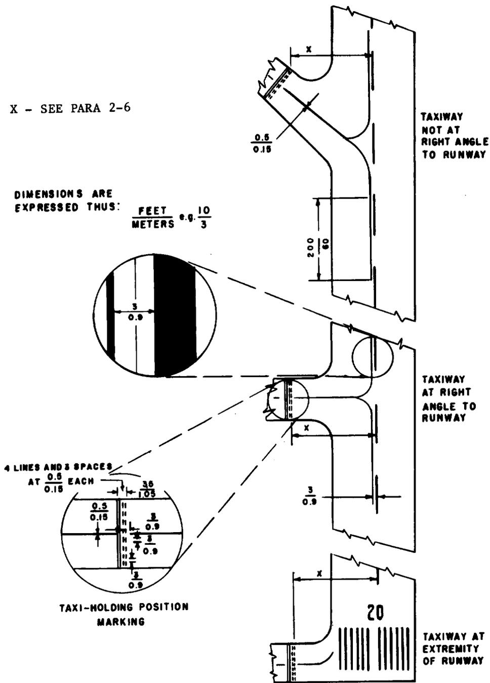
Figure 2-6. Taxiway/runway intersection marking. (Sheet 1 of 2).
