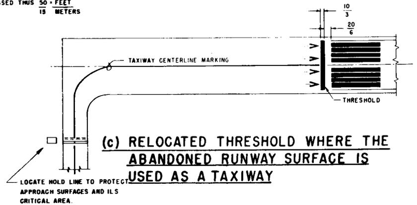
**(c) RELOCATED THRESHOLD WHERE THE ABANDONED RUNWAY SURFACE IS USED AS A TAXIWAY**
