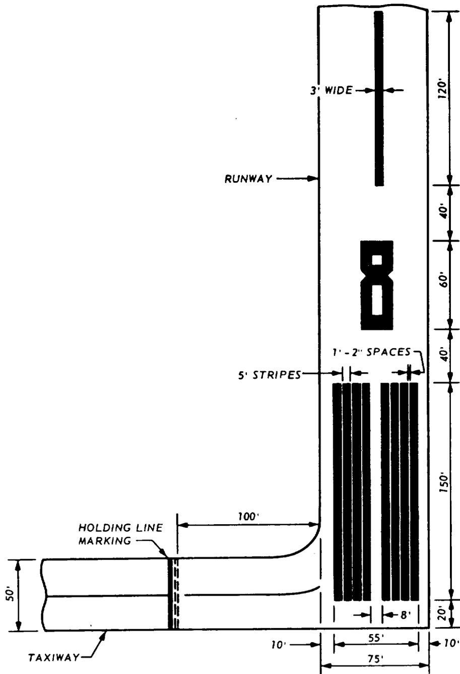
Figure 2-2. Precision instrument runway marking. (Sheet 2 of 2).
